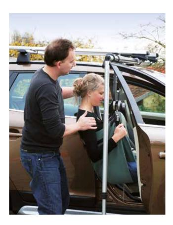
A portable lifting aid, which is fixed to a pair of Thule carriers (not included) on a vehicle with roof railing. The passenger is lifted by a self-locking lift mechanism and moved in or out of the vehicle by sliding along the vertical bar, which is fixed to the roof rack. When the lift procedure is ready, the vertical bar and the support pillar are stored inside a tube on the roof rack.
